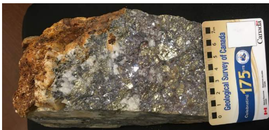
Photo 2: Sample No. Y738503 from Q19 vein; 202 g/t Au, 1,735 g/t Ag and 32.1% Pb
